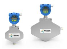
TRICOR's U-Shape Coriolis Mass Flow Meters range in flow rate from 5500 to 230,000 kg/hr (202-8450 lb/min) and withstand pressures up to 1450 psi (100 bar). The TCM 5500 is rated at a maximum pressure of 5,000 psi (345 bar). These meters have good overall accuracy, zero stability, and pressure drop. The simple self-draining U-shape tube design provides for easy cleaning/flushing.
